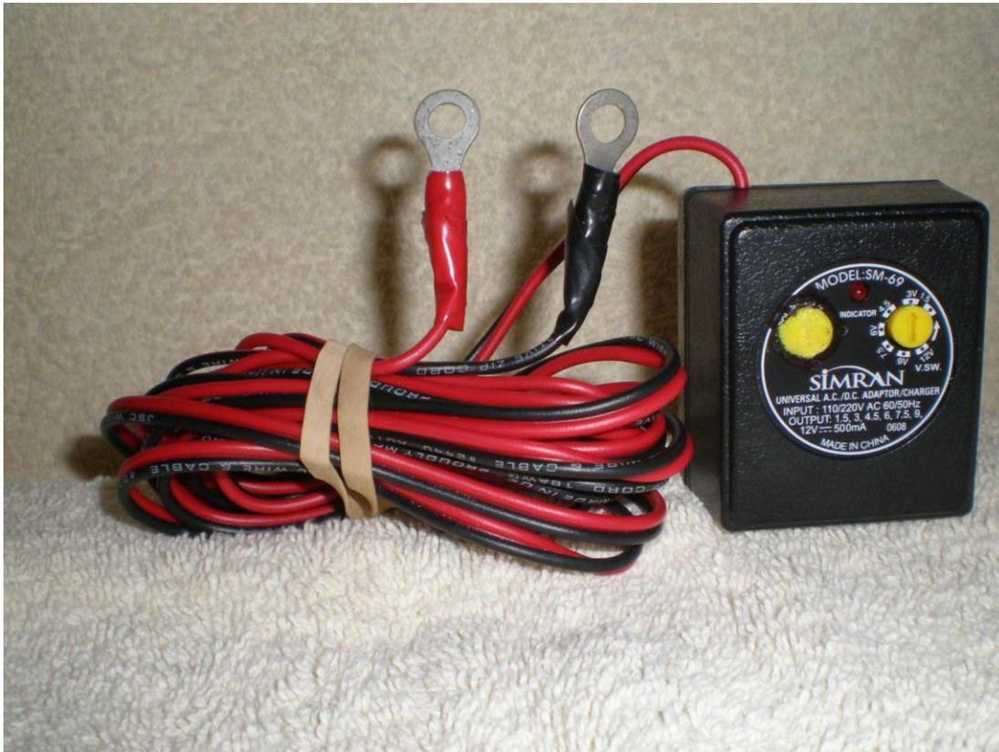
Care must be taken not to short circuit the red and black leads from the power supply; (it will burn out the windings in the power supply.) This power supply is intended for indoor usage only..
